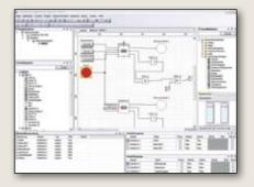
The IndraWorks Machine Simulator add-on simulates the I/O peripherals of automation systems, extending the range of simulation tools for the IndraLogic and IndraMotion control systems from the Rexroth Automation House. Additional Rexroth simulation tools with the IndraWorks Machine Simulator include IndraWorks View3D for 3D machine animation and the VAM Simulator for virtual machine or simulation operation. www.boschrexroth.ca
