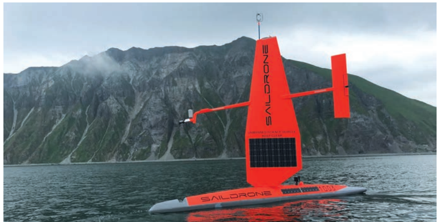
Designed and manufactured by California-based Saildrones, these wind and solar-powered autonomous surface vehicles, equipped with echosounder sonar, perform bathymetric surveys in the Bering Sea.
