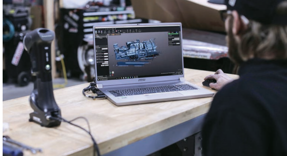
To help design his drift racecar's hand control system, Parsons used a Creaform 3D scanner to create a CAD model of this T-56 manual transmission.
