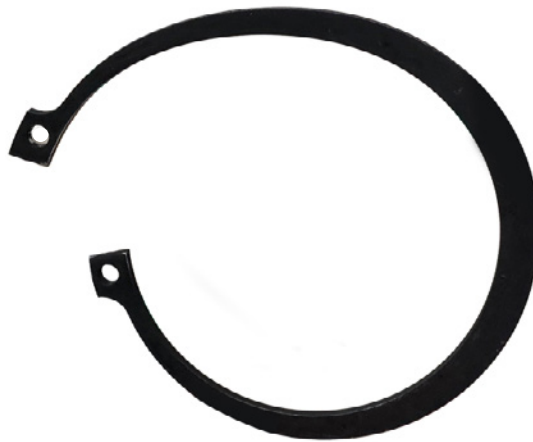
Fig 11. Yielding (deformation) on a snap ring after use at high RPM.
