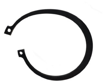
Fig 4. Yielding (deformation) on a Tapered Section Retaining Ring from rotation.
