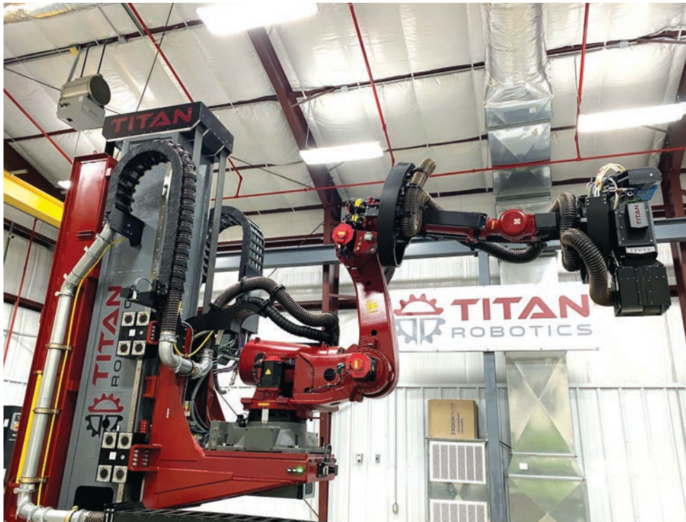
Developed by Titan Robotics, this depainting system employs continuous-wave lasers to burn paint off an airplane's surface, which reduces workers' exposure to toxic chemicals.
