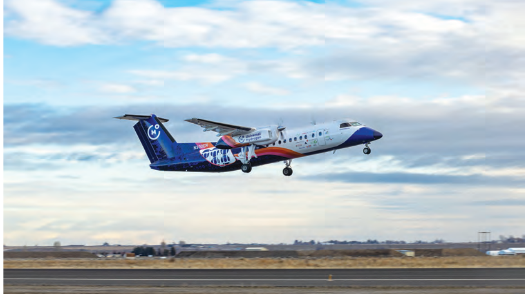
Universal Hydrogen's modified Dash-8, nicknamed "Speedy McClean," successfully completes first flight of a hydrogen-powered regional airliner.
