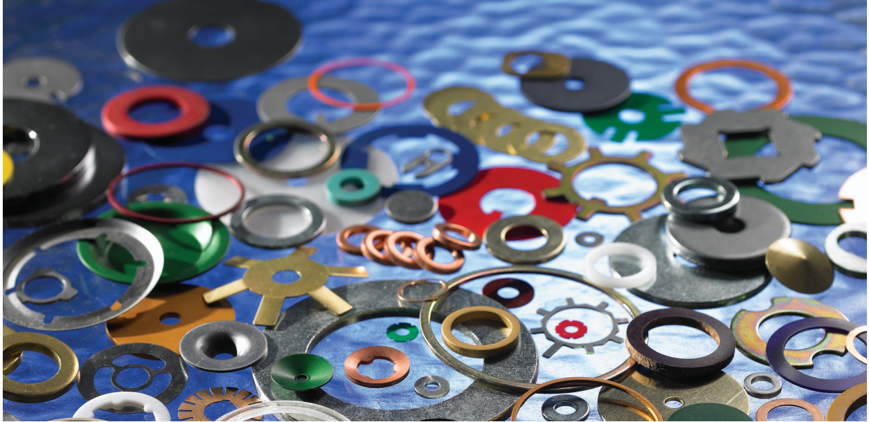
Stampings and washers available in a complete range of sizes up to 12" x 12" (flat) with thickness ranging from .005" to .190" (varies by material) and draws up to 3" deep and 8" in diameter.
